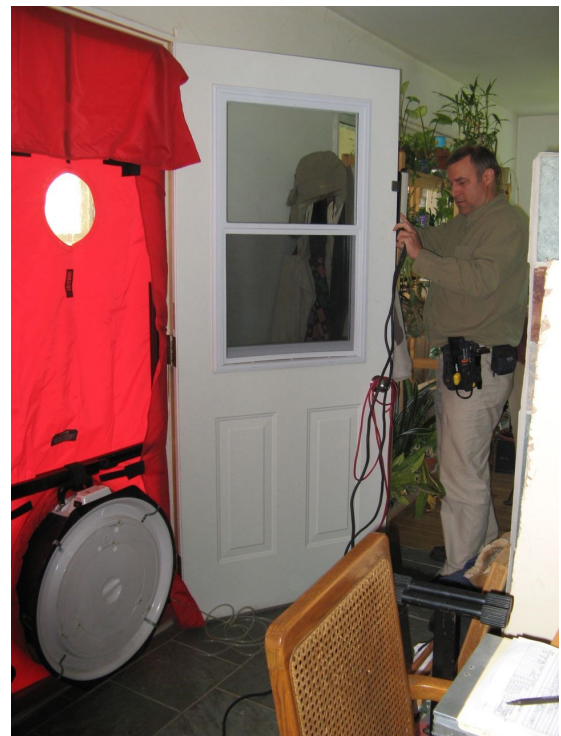
Al Leonard, licensed energy advisor, performing a blower door test.
